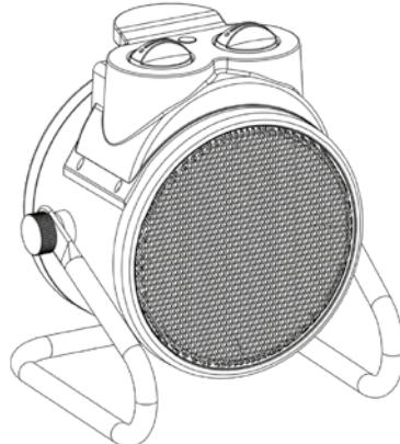
Make a minimum distance of 1m from any item to the air inlet and outlet to allow a good circulation of the airflow.
